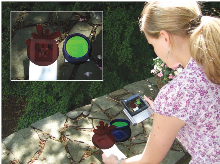
Figure 2. Augmented view of a basic interaction technique: putting two markers next to each other in the game The Alchemists .
