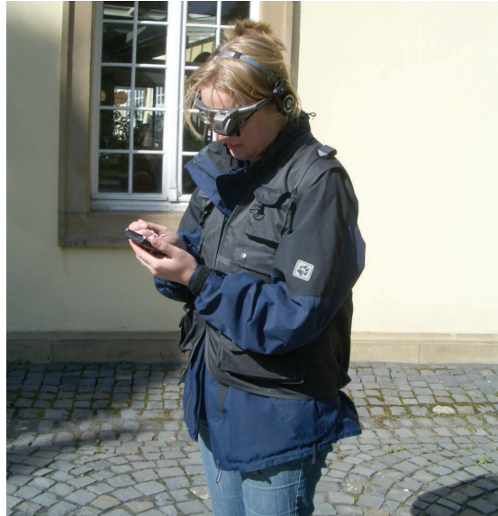
Figure 4. The TimeWarp mobile AR system including an AR jacket, a PDA, headphones, and a head-mounted optical see-through display.
