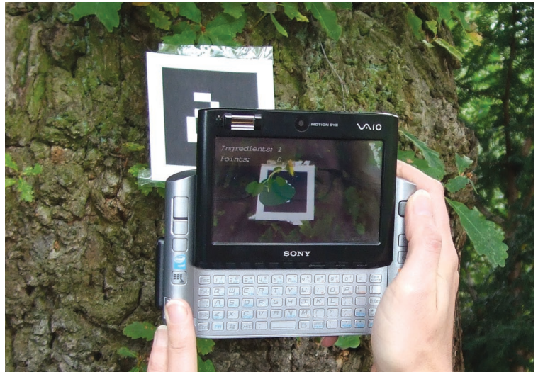
Figure 1. Ultramobile PC used as a Magic Lens in the game The Alchemists . The Magic Lens augments the real environment by applying virtual objects to fiducial markers.
